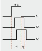
Total current consumption is equal to the power consumed by the solenoid pilots plus the current consumed by the electronics controlling the bases. To simplify the calculation, you can consider 3.2W consumed by each solenoid pilot simultaneously and 0.3W by each active solenoid pilot.
